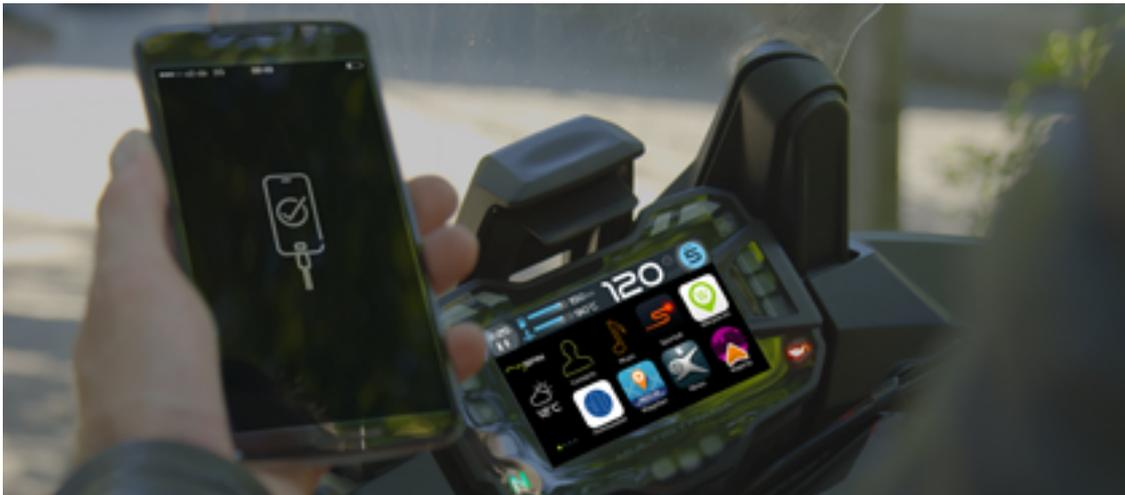
Figure 3-4: Launcher App in connected mode (left) and home screen on instrumental cluster home screen (exemplary design)
